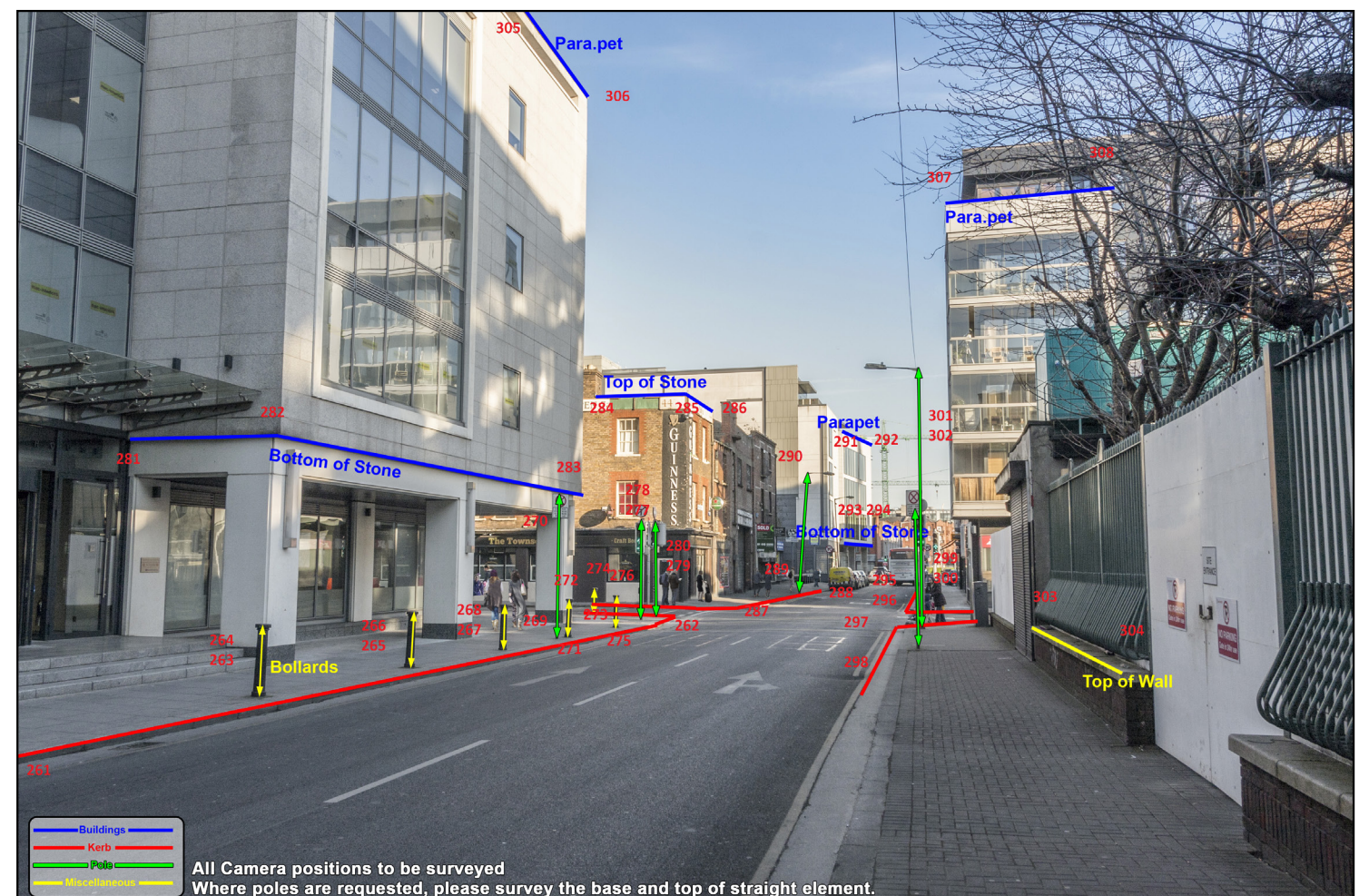
Fig.8: Fixed reference points fully surveyed and numbered.
